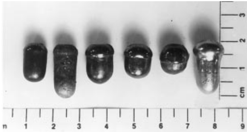
Figure 2. Illustration of the growth of a 'head' on the iron ingot with time caused by dissolution of the CaO crucible along its line of contact with the slag-metal interface. Desulphurization times increase in passing from the ingot on the left to the ingot on the right.
